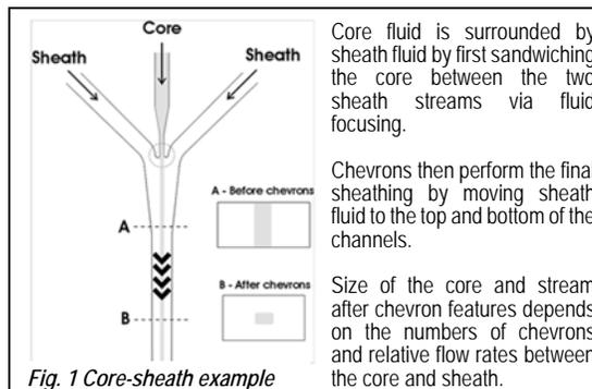
Fig. 1 Core-sheath example
