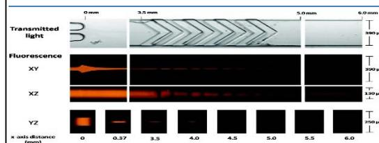
Fig. 2 Images of the sheathing process. Core, with dye, is initially sandwiched between two sheath streams (0 to 3.5mm). Entry into chevrons (3.5 to 5mm), core height is much reduced as sheath surrounds core. Tight core stream enters interrogation zone (6.0mm). Core to sheath velocity in this example is 10 to 400  $\mu$ L/min.
