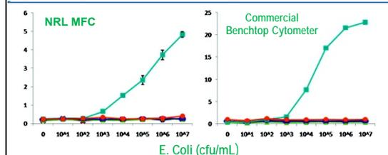
Fig. 4 Multiplex Immunoassays. Abstracted data from dose response curves from a 6-plex assay for 3 bacteria (E. Coli, Listeria, Salmonella) and 3 toxins (cholera, SEB, ricin). Data from the NRL microflow cytometer is compared to an analyses using a commercial benchtop flow cytometer and approaches comparable sensitivity. Kim, JS et al, 2009. *Analyt. Chem.*, 81, 5426-5432
