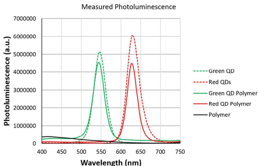
**Figure S3.** Raw measured photoluminescence (PL) data for red and green QDs before and after incorporation into thiol-yne polymer matrices. PL for thiol-yne polymer also indicated in the plot as ‘polymer.’
