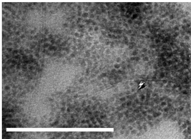
**Figure S2.** Representative TEM image of red QDs (1.5  $\mu$ M) within a thiol-yne nanocomposite. Scale bar represents 200 nm.
