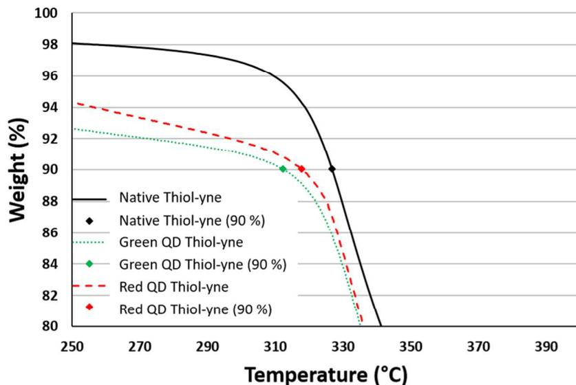
**Figure S4.** Thermal gravimetric analysis plots indicating the temperature at which 90 wt% of the polymer remains.
