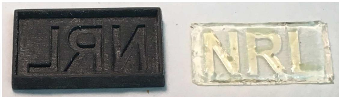
**Figure S1.** Figure showing the reverse mold (left) used to form the 'NRL' polymer (right) that was composed of both native thiol-yne polymer and red QD thiol-yne nanocomposite.
